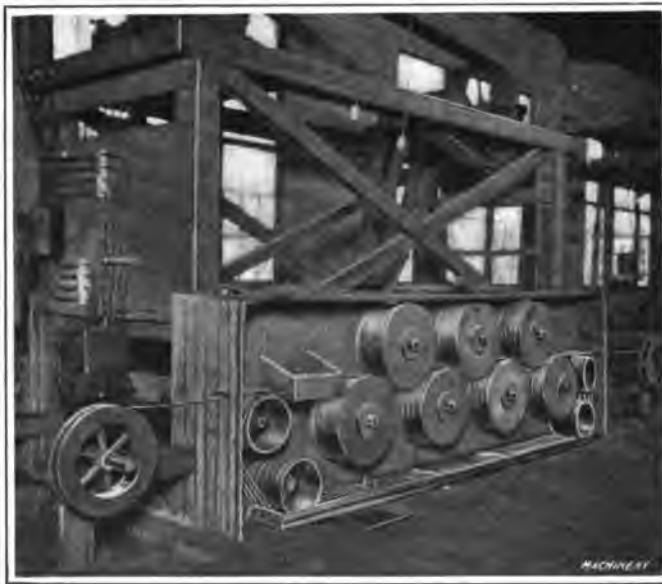
Fig. 21. Special Polishing Machine designed for Applying High Finish to Strip Steel
